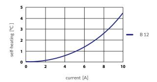
The characteristic curve in the diagram is measured with a thermal switch without any insulation in an oil bath.
