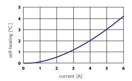
The characteristic curve in the diagram is measured with a thermal switch without any insulation in an oil bath.
