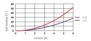
The characteristic curve in the diagram is measured with a thermal switch without any insulation in an oil bath.
